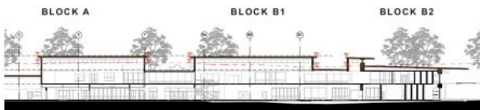
Figure 4 Extract of long section which shows the variation of height with respect to Blocks A, B1 and B2. Natural ground level shown in the red dashed line.
